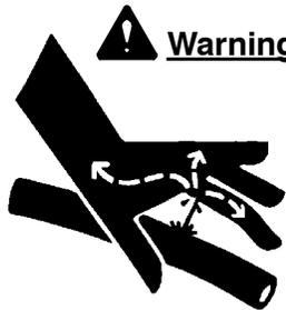
**⚠ Warning:** Escaping fluid under pressure can penetrate the skin causing serious injury. Avoid the hazard by relieving pressure before disconnecting hydraulic lines. Tighten all connections before applying pressure. Search for leaks with a piece of cardboard. Protect hands and body from high pressure fluids. If an accident occurs, see a doctor immediately. Any fluid injected into the skin must be surgically removed within a few hours or gangrene may result.
