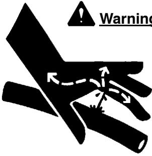
**Warning:** Escaping fluid under pressure can penetrate the skin causing serious injury. Avoid the hazard by relieving pressure before disconnecting hydraulic lines. Tighten all connections before applying pressure.
