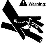
Warning: Escaping fluid under pressure can penetrate the skin causing serious injury. Avoid the hazard by relieving pressure before disconnecting hydraulic lines. Tighten all connections before applying pressure.
