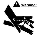
Marning: Escaping fluid under pressure can penetrate the skin causing serious injury. Avoid the hazard by relieving pressure before disconnecting hydraulic lines. Tighten all connections before applying pressure. Search for leaks with a piece of cardboard. Protect hands and body from high pressure fluids.
