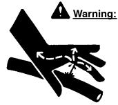
Warning: Escaping fluid under pressure can penetrate the skin causing serious injury or death. Avoid the hazard by relieving pressure before disconnecting hydraulic lines. Tighten all connections before applying pressure.
